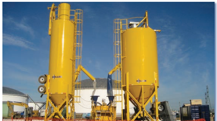
A soil mixing grout slurry batch plant. Real-time monitoring of all mixing parameters allows for control of batching and pumping operations.
