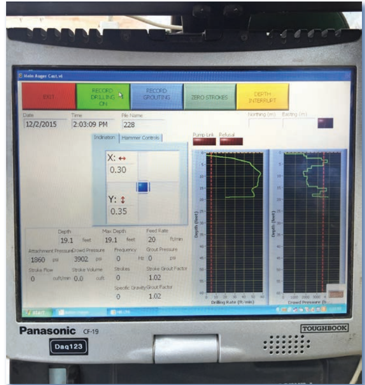
In-cab DAQ monitor displaying real-time quality control feedback during RI construction.
