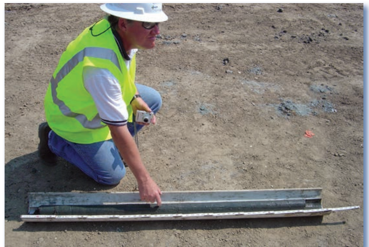
Fresh core sample ready for curing and subsequent strength testing.
