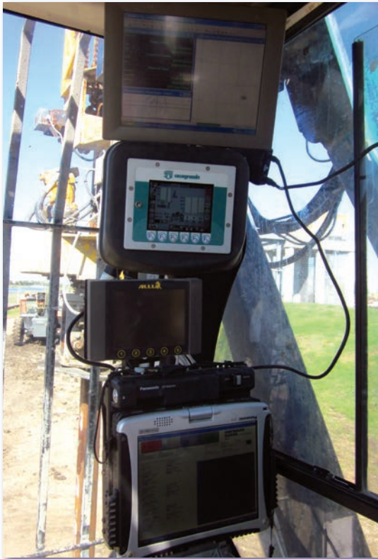
The in-cab monitor displays data such as binder and tool depth, alongside specified target values.
