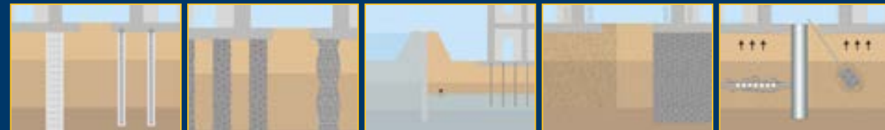
Deep foundations Ground improvement Groundwater control Liquefaction mitigation Releveling structures
