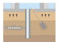
Releveling structures is achieved by either lifting through a direct connection to the structure or by injecting grout at depth to raise both the overlying soil and the structure it supports.
