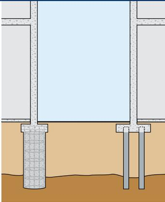
Heavy foundations are structural elements that transfer loads through soils with insufficient strength and/or stiffness to underlying competent soils or rock.
