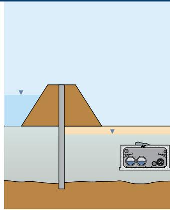
Seepage control involves the construction of barriers in soil and rock, sealing below-grade structures to restrict the movement of water, or dewatering for excavations.
