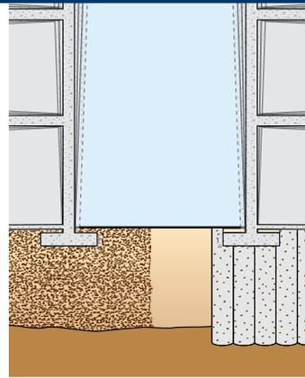
Liquefaction mitigation is achieved by densifying loose granular soils or constructing subsurface reinforcements to resist seismic forces.
