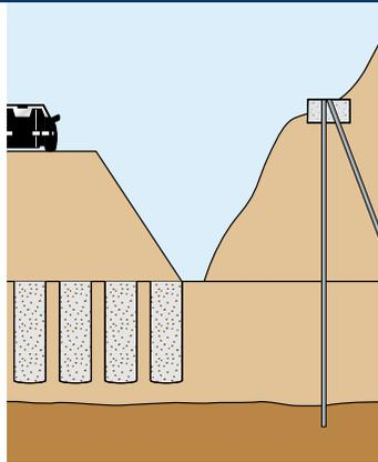
Slope stabilization involves the strengthening, reinforcing, or supporting of soil slopes to produce a sufficient stability factor of safety.
