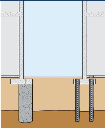
Underpinning provides additional support to existing foundations that are unable to safely support existing or additional planned loads or that experience reduced support.
