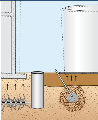
Releveling structures is achieved by either lifting through a direct connection to the structure or by injecting grout at depth to raise both the overlying soil and the structure it supports.
