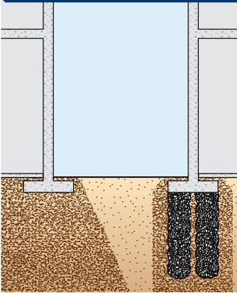
Bearing capacity/settlement control involves modifying soil properties or reinforcing the soil to achieve a designed performance.
