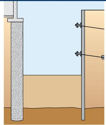
Excavation support involves retaining soil whose stability is impacted by a man-made excavation or fill. Existing adjacent structures may also require support.
